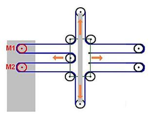
Fig. 2. Layout of the machine work
