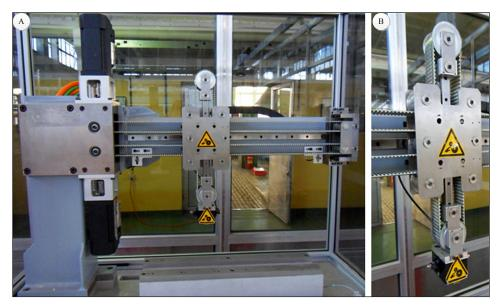
Fig. 1. The automated station with complex kinematics; A) external appearance B) actuator
